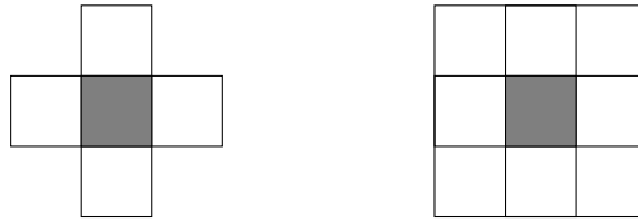
Figure 13: Commonly-used neighbourhoods for Cellular Automata: Von Neumann neighbourhood (left) and Moore neighbourhood (right)
